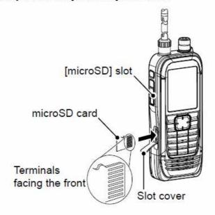
CAUTION: DO NOT forcibly or inversely insert the card. It will damage the card or the slot.
